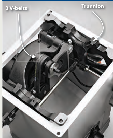
The trunnions on this Steel City saw, as well as on Craftsman's hybrid, mount to the cabinet rather than the top.
