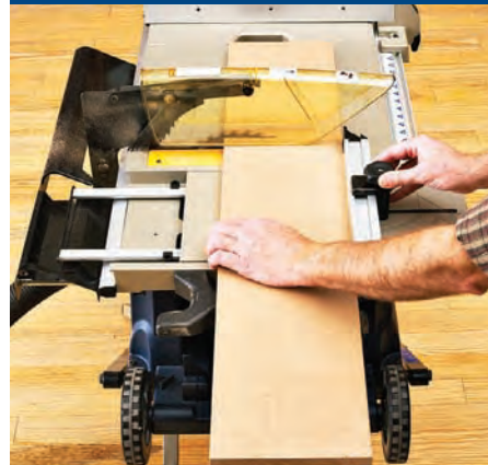
Ryobi's job-site saw features a sliding crosscut table that locks into place when you want to make a rip cut or for storage.
