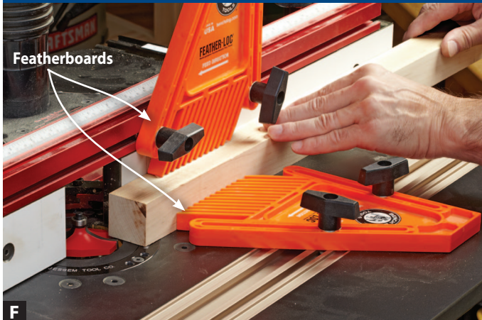
F A featherboard's slanted fingers resist any backward forces, helping you maintain control of a workpiece even if kickback occurs.
