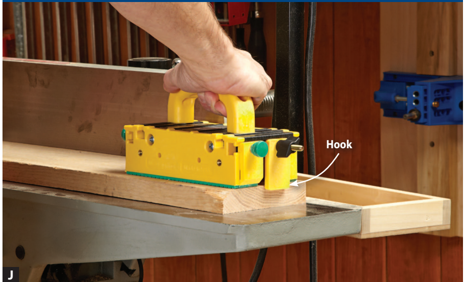
Whether it's purchased or shop-made, a pushblock that hooks the rear end of the workpiece helps you keep the board moving forward across the jointer while also keeping it firmly against the table.
