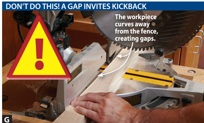
G With gaps behind the cutline, the rotation of the blade can shift the workpiece backward, pinching the blade.
