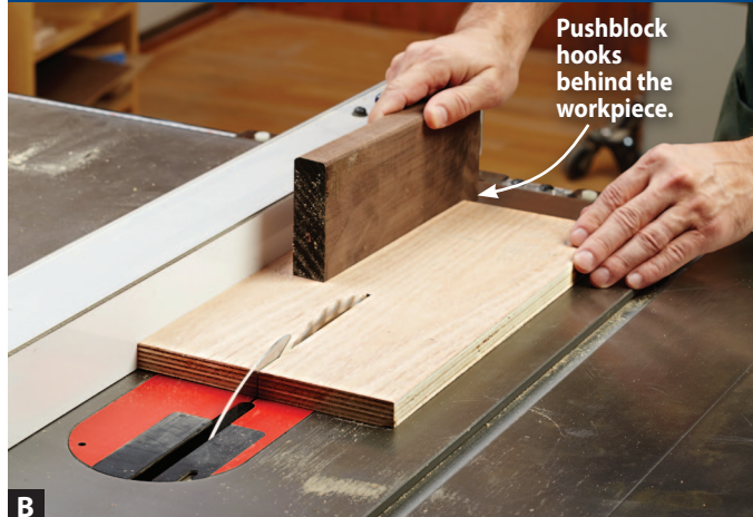
B A long notch in one edge of a scrap creates a hook that helps you push the workpiece down, forward, and against the fence.
