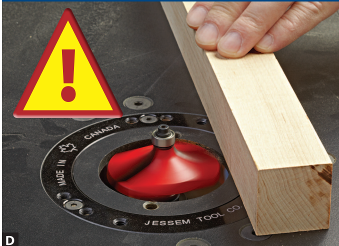
D With no way to control the workpiece or cutting depth once the wood contacts the cutters, the rotation of the bit will jerk the workpiece violently.
