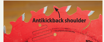
The shoulder behind each tooth on this 24-tooth rip blade limits how deeply the next tooth will cut.
