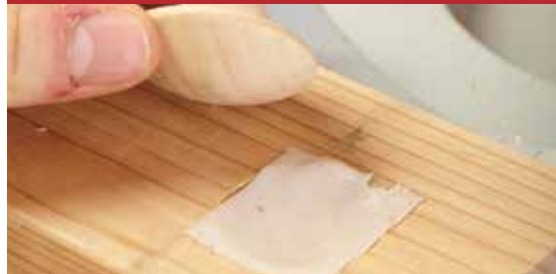
In scrap, drill a shallow hole, cover it with double-faced tape above left , and press the knob into the hole. Clamp the scrap beneath the bit and drill slowly.
