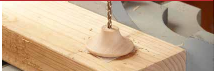
In scrap, drill a shallow hole, cover it with double-faced tape above left , and press the knob into the hole. Clamp the scrap beneath the bit and drill slowly.
