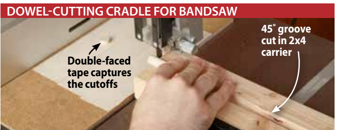
Build this carrier with the 2x4 extending just past the blade; then, run it through to cut it flush and provide a reference edge for aligning cutlines on the dowel.
