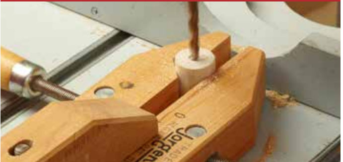
A V-shaped notch bandsawn into one jaw of a handscrew captures a dowel, keeping it from spinning during drilling.
