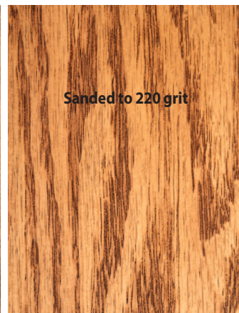
Sanding this board to 220 grit eliminates unsightly scratches.
