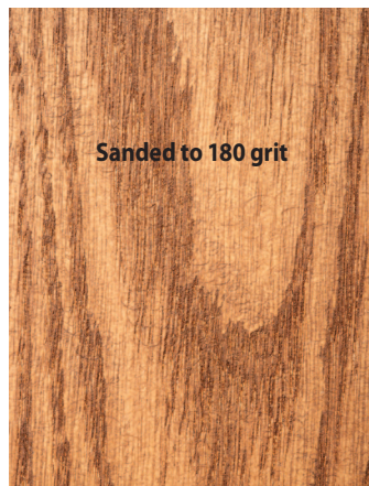
This oak board, sanded to 180 grit and stained, reveals swirl marks.
