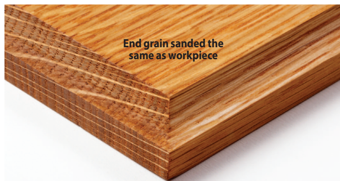
This end grain, sanded to 220 grit like the rest of the workpiece, soaked up more finish and looks darker than the face and edge grain.
