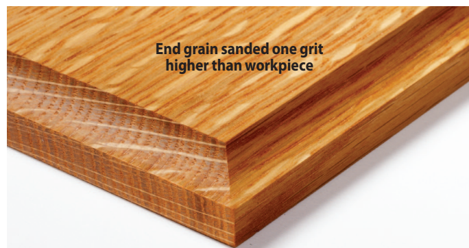
By sanding only the end grain to 320 grit—but stopping at 220 for the face and edges—the end grain's color better matches the overall tone.
