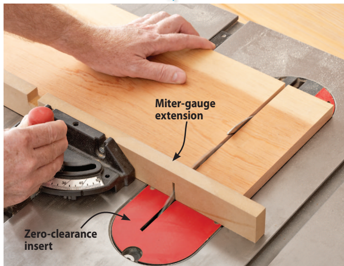
Make custom zero-clearance inserts for different blade angles and setups, such as beveled cuts and dados.
