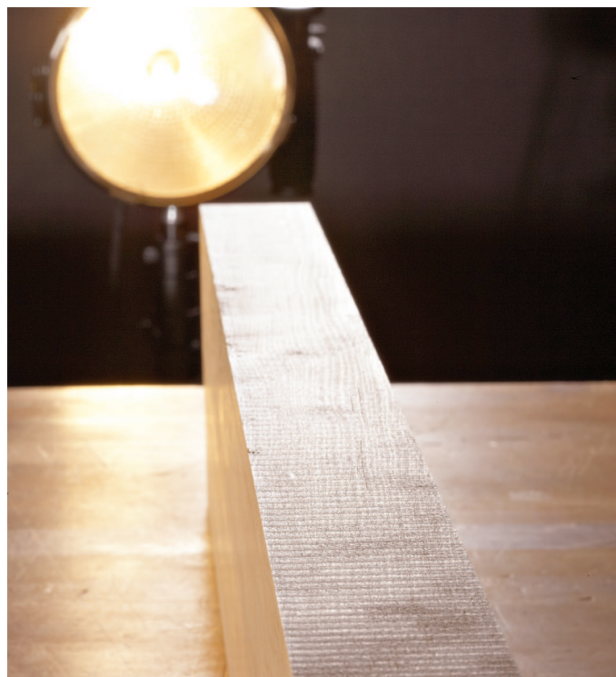
A low-angle raking light reveals scallop marks left on this board's edge by a jointer's straight-knife cutterhead.
