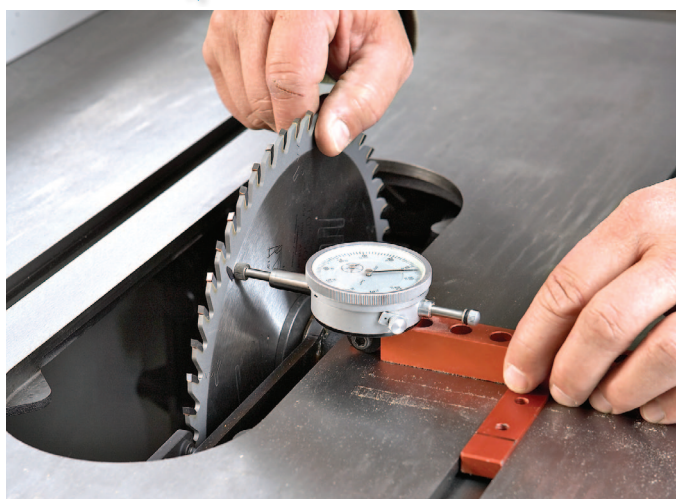
To align a tablesaw top to the blade, adjust it until a dial indicator (or combination square) reads the same at the front and back of the blade.
