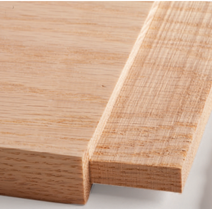
This tenon, cut with a tablesaw dado blade, retains subtle ridges that will impede the joint's glue adhesion.
