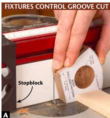
A With a stopblock and feather board in place, cut a groove in each side of the body (A). Slide your hand on top of the fence for safety.
