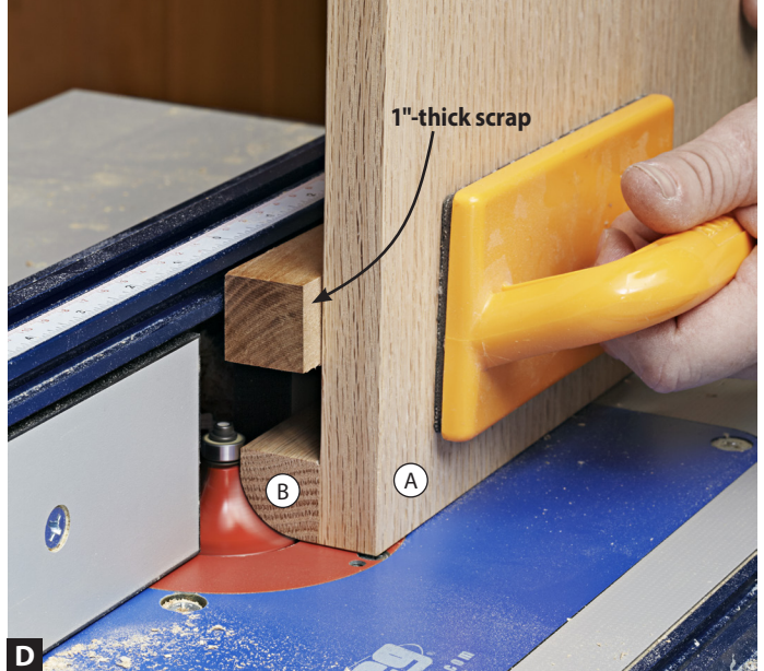
D Attach a piece of 1"-thick square scrap to the body (A) with double-faced tape to keep the bench hook parallel to the router table fence.
