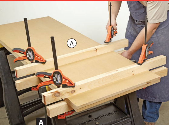
Distribute clamping force evenly across the tops (A) by clamping pairs of leg blanks side by side and spaced evenly along the MDF panels.
