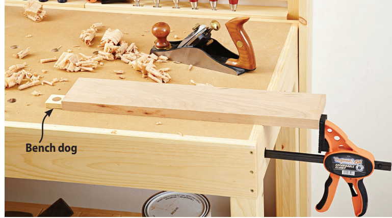
Clamp a board in place against a bench dog (Shop Tip, page 28) for easy face-planing, chiseling, or sanding. See page 27 for details on the clamping blocks, mounted beneath the benchtop.
