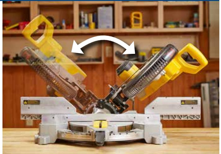
Most miter saws, like the one above, have a motor/blade head that tilts in one direction to provide compound-cutting action with the table/head rotated at an angle. Dual-bevel saws, like the one at right, tilt both left and right, making it easier to cut large and bulky workpieces with less repositioning.
