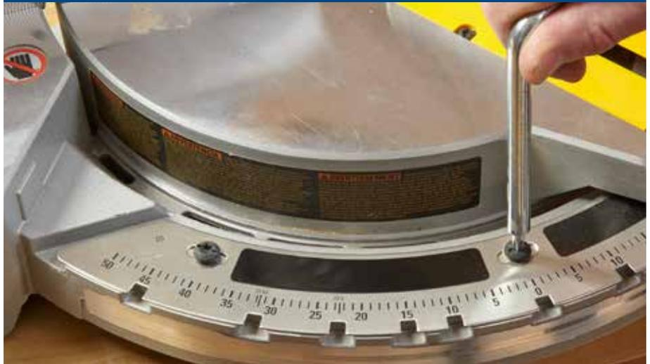
For the ultimate in convenience and spot-on accuracy, seek a saw—like this DeWalt—with a miter scale that adjusts by simply loosening a few screws with an onboard driver.
