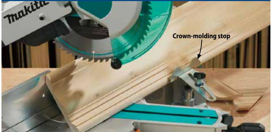
To quickly and reliably position crown molding at the correct spring (installed) angle, secure crown-molding stops like this one to the saw's hold-down attachment holes.
