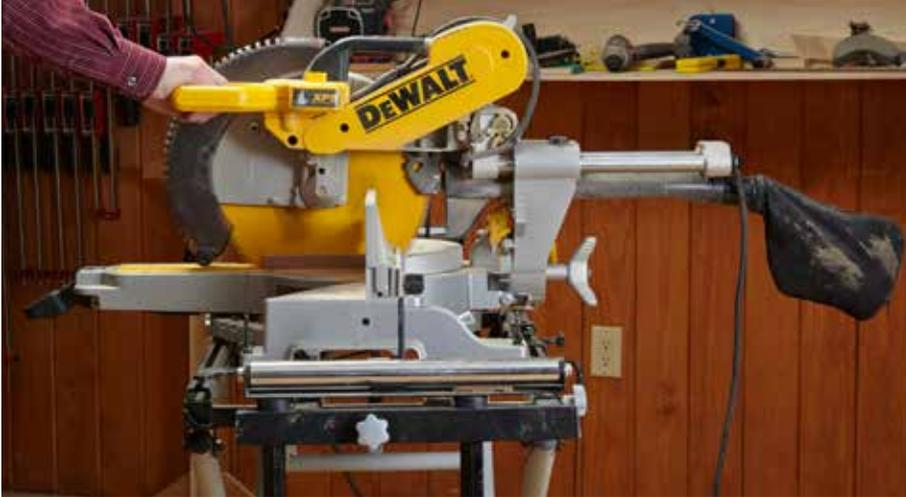
You'll need up to a couple feet of extra room behind a sliding miter saw to accommodate its sliding mechanism and dust bag. Consider that if you plan to place the saw against a wall.
