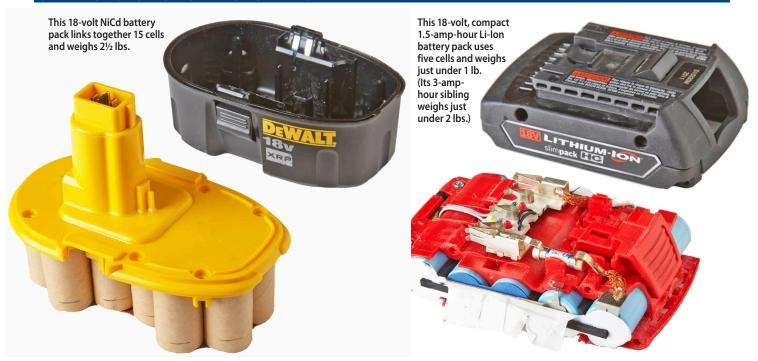
Then, in the early 2000s, manufacturers turned to lightweight lithium-ion (Li-Ion) technology, which had proved itself in laptop computers, cellular phones, and other electronic products. Li-Ion enabled manufacturers to chop
