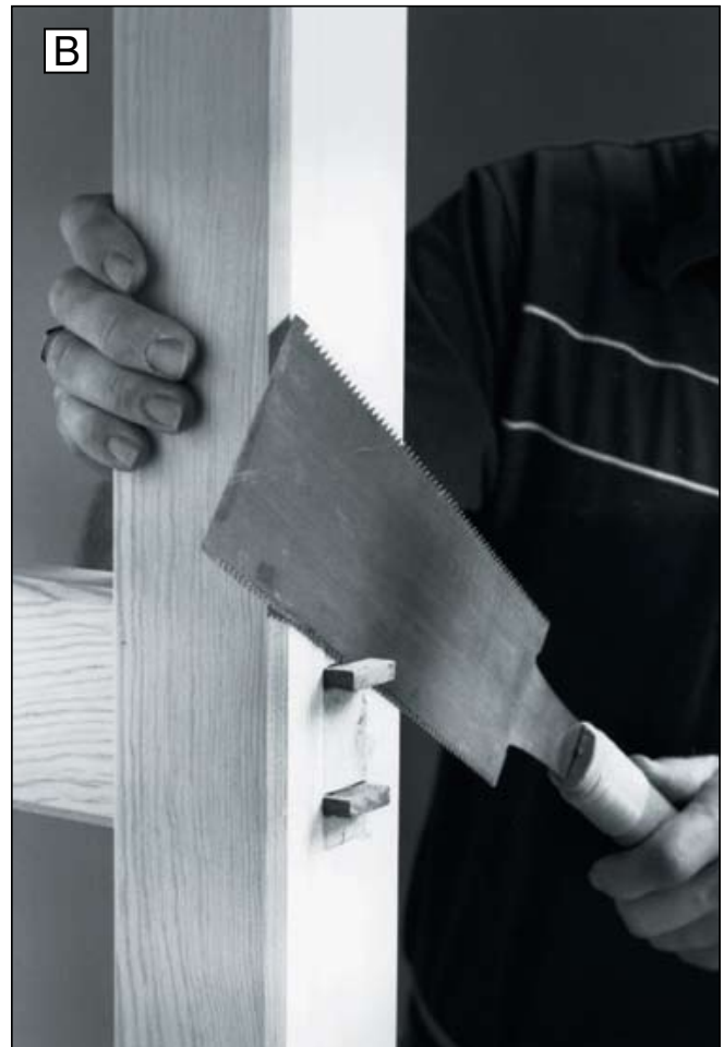
Tap the hardwood wedges into the notches. After the glue dries, trim the wedges flush with the legs.
