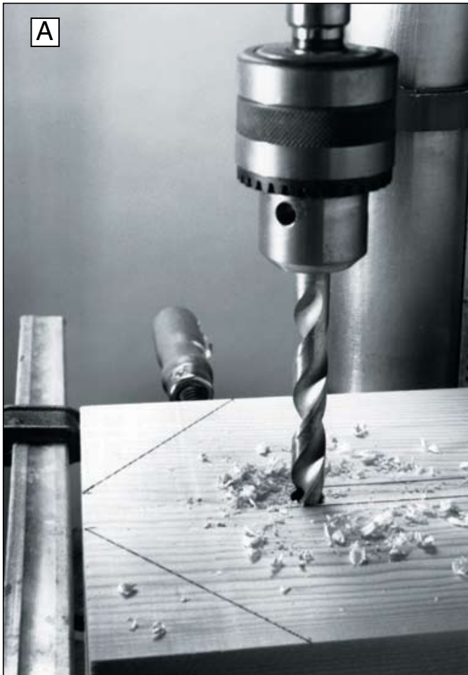
Clamp the feet together, and drill a 1/2" hole at the marked centerpoints to form the radiused bottoms.
