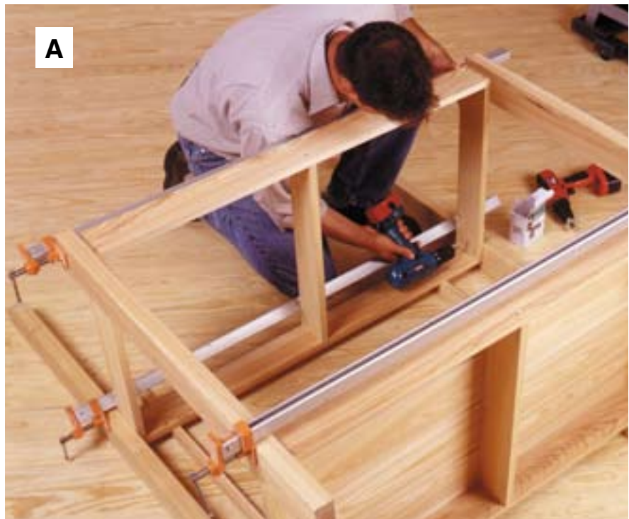
Drill countersunk shank and pilot holes, then drive 2" deck screws through the frame assemblies into the legs.
