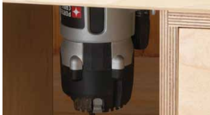
A good table-mounted router makes bit changes hassle-free. An angled wrench to hold the spindle sure helps.
