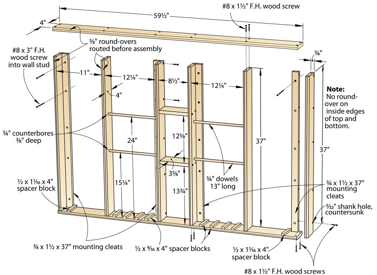
It may not be apparent at first glance, but this simply constructed wall-mounted unit can store an assortment of 90 clamps. Made from inexpensive pine, it offers shelves and dowels for organizing anything from
