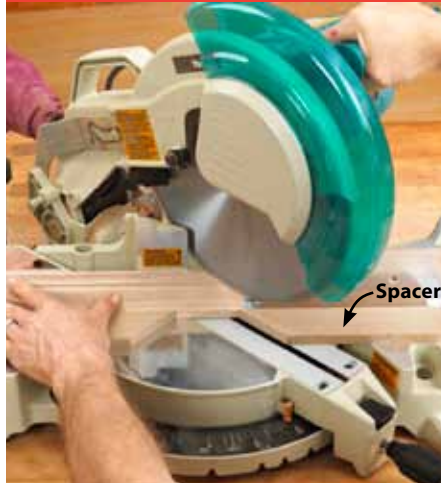
When the crown molding doesn't extend along one side of the crown molding stop, add a spacer there to keep the spinning blade from moving the stop.
