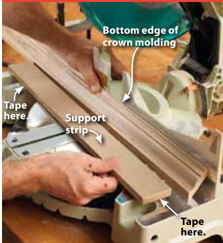
When attaching the crown molding stop strip, apply double-faced tape so it adheres to the fixed outside edges of the miter saw table, not the rotating part.
