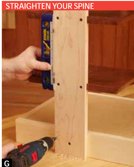
G Using the single screw as a pivot point, plumb the spine. Then drill and drive four more screws to secure the spine in position.
