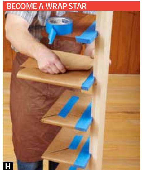
H Carefully mask each shelf near the spine, before wrapping the entire shelf with kraft paper, overlapping the masking tape.
