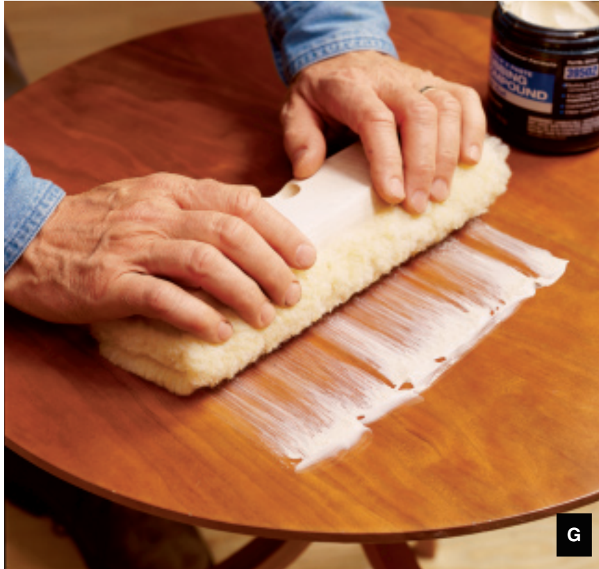
A lamb's wool applicator like the one shown here gives you room to grip with two hands and apply pressure as you rub. The rubbing agent being used on this tabletop is a fine automotive compound.
