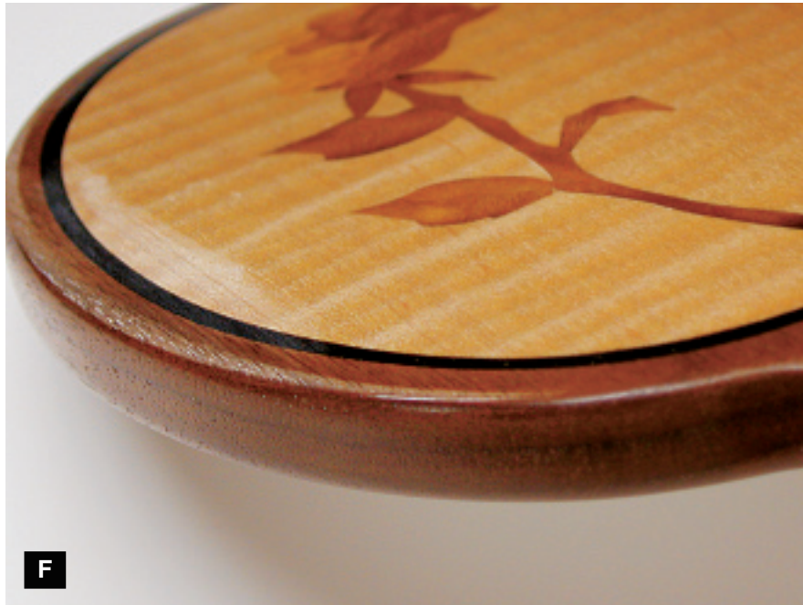
F When you don't have much finish to work with, it's all too easy to rub through it and expose the bare wood, as shown here on a handheld mirror.
