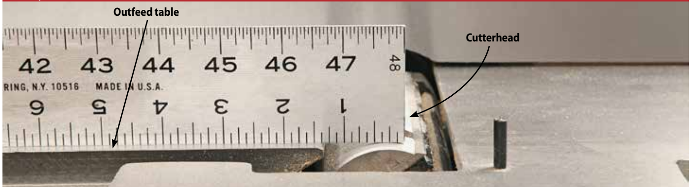
Set the outfeed table flush with the cutterhead, then check for gaps between the straightedge and table.
