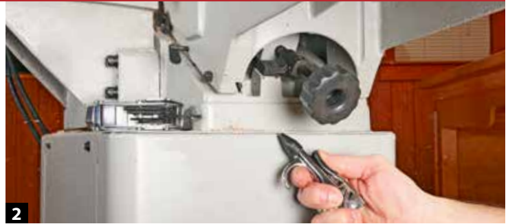
2 Lift the end of the table to allow the solvent to reach all areas. Force out any remaining grease and grime with compressed air.
