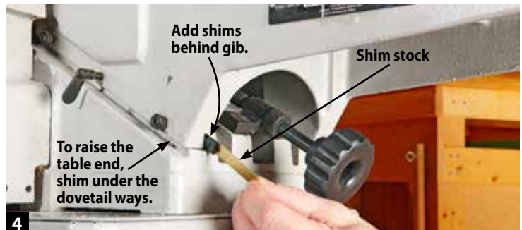
4 Cut .005 brass shim stock ( Source ) as long and wide as the gib, grease the shim, and slide it behind the gib. Add additional shims if needed.
