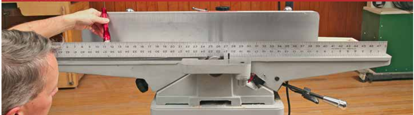
Shine a flashlight behind a straightedge to highlight gaps that require you to make adjustments.
