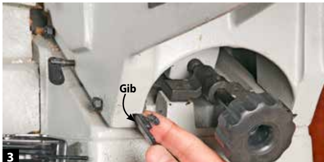
3 Slide the gibs (metal bars between the dovetail ways) out partially and apply a liberal coat of lithium soap grease; then reinsert them.
