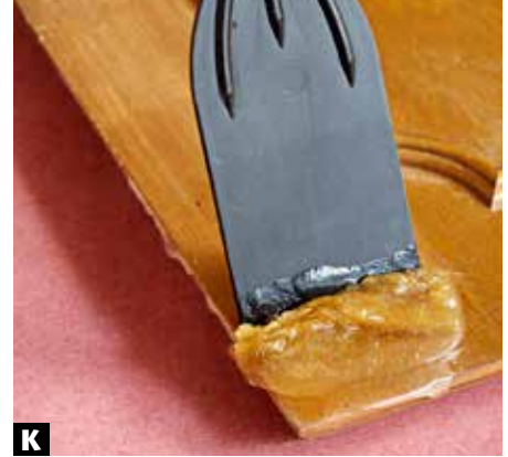
K Unlike sanding, chemical stripper dissolves the finish even down inside the pores of the wood, making it easier to stain.
