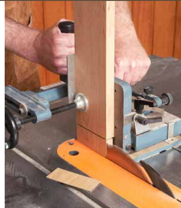
Set your tenoning jig so the tenon-cheek offcut falls away from the blade, not trapped between the blade and jig.
