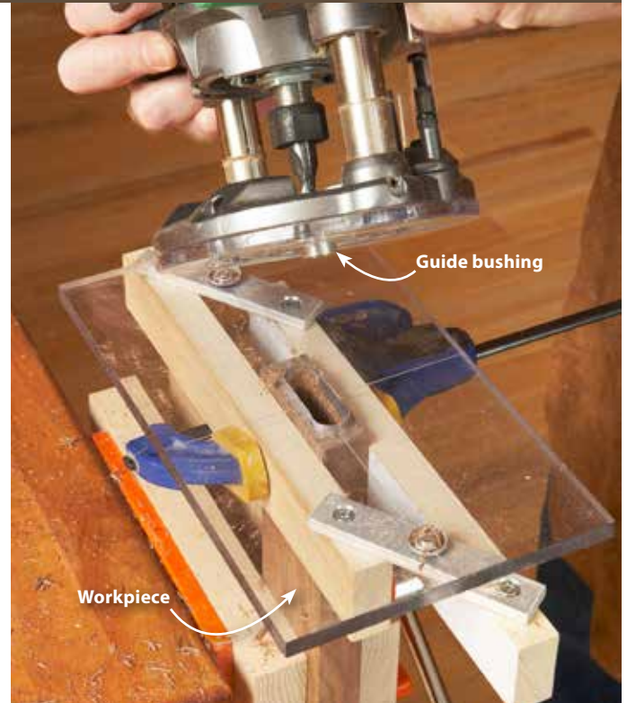
END GRAIN: A mortising jig provides a large, stable surface for the router when routing mortises into the ends of workpieces.
