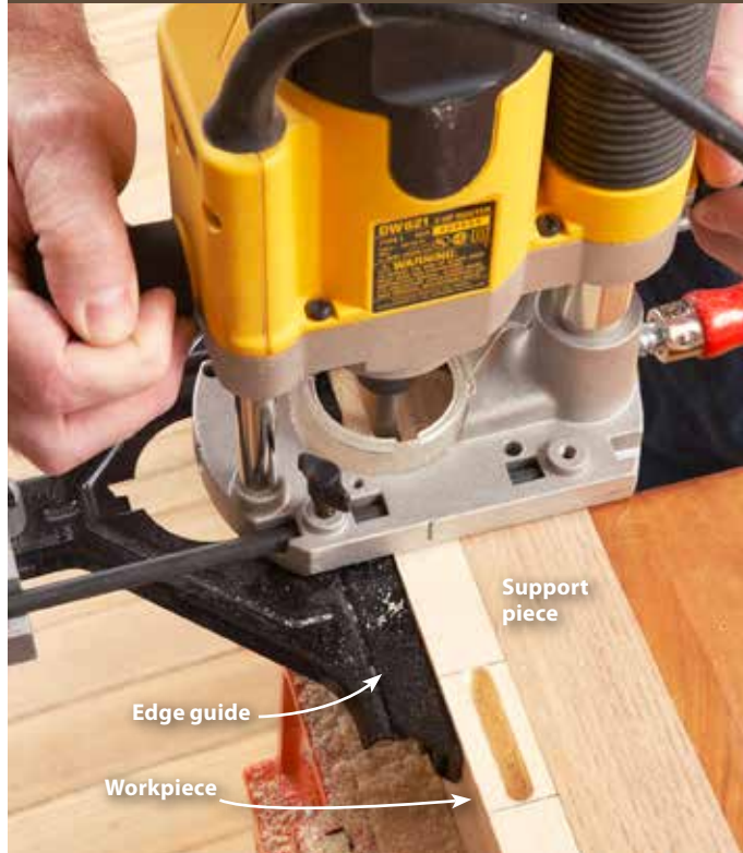
EDGE GRAIN: For narrow workpieces, such as this stile, clamp an auxiliary support piece to it to prevent the router from tipping.
