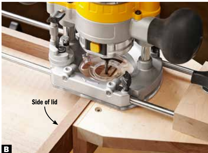
B A downcut spiral bit cuts clean shoulders and leaves a rounded end that matches the hinge leaf. An edge guide keeps the router on track while routing the recesses.
