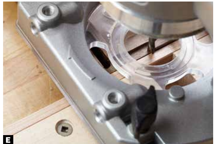
C Starting \frac{1}{8} " from the rear edge of the lid or box, rout a \frac{5}{8} "-long mortise inside the existing recess. Rout in several successively deeper passes.
