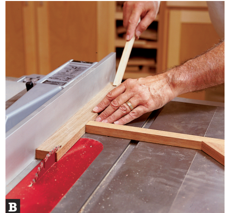
B If one pass won't produce enough spline stock, clamp a stop to the table before ripping. Slide the fence between cuts to set the board against the stop.
