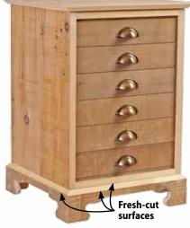
Here's the chest with the fresh-cut edges and ends. Note how the drawer fronts appear darker than the sides—reclaimed stock can vary greatly.
