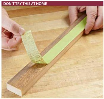
Masking tape will lift old finish from the face grain. You're better off carefully applying stain to fresh-cut edges/ends with a brush and a steady hand.
