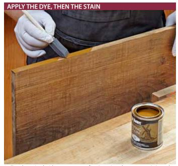
Aniline dye, mixed with water, goes on first (opening photo, page 46). Once the dye has dried, apply the chosen stain (above) and wipe off the excess.
