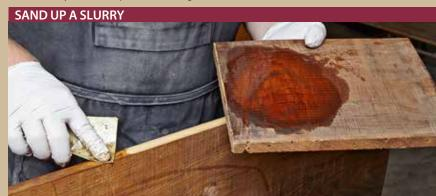
Apply some thinned oil-base natural-tint stain and loosen up the old finish by sanding in a circular motion. Add more stain and keep sanding until you've created a rich slurry that you can apply to the raw edges with the same piece of sandpaper.
