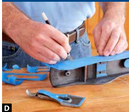
D Mask areas not getting paint; then use a craft knife to precisely trim the tape. Cut from the center, out, drawing the blade along the iron.
