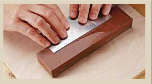
The Naniwa fine-grit ceramic stones dished out so rapidly we had to stop and flatten them often. Not doing so would produce rounded tool edges.
