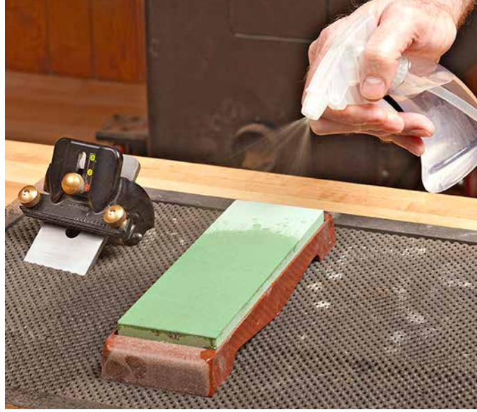
Even if they're fully dry, you need only give ceramic stones a quick spritz of water before sharpening tools.
