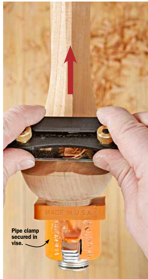
Give it a push on end grain. Gripping a low-angle shave near the blade, push the tool down and away for end-grain cuts, such as this cabriole-leg foot.
