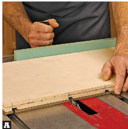
A After cutting dados in the plywood base, glue the hardboard to the dadoed face. Mount the two outside blades of a dado set in your tablesaw, and cut slots through the hardboard centered over each dado.
