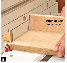
routing them, here's a way to hide the mortise edges beneath the lip of a rabbeted tenon for a clean look. To start, mark your workpiece to show the mortise ends and centerline.
