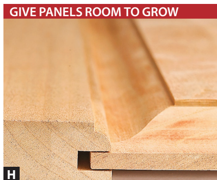
H When sizing a solid-wood panel to fit within a frame, allow about 1/8" between the edge of the panel and the groove bottom.
