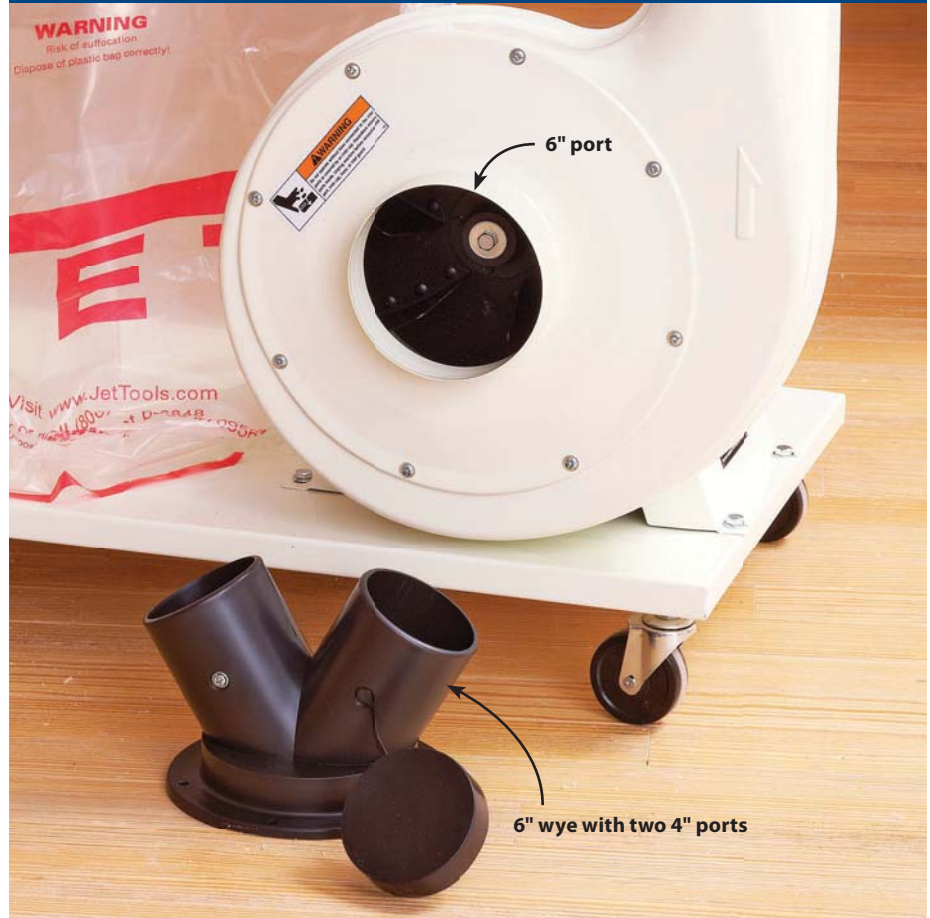
Instead of connecting a hose to each 4" port, increase the dust collector's airflow by connecting ductwork that matches the larger-diameter port hidden behind the wye.
