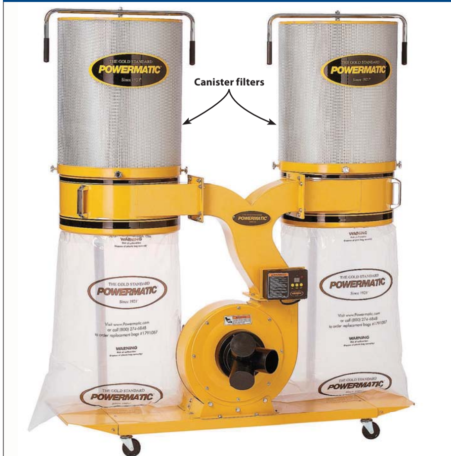
This 3-hp, single-stage collector features two canisters that provide double the filter area of a typical single-stage collector, while two lower bags increase chip-holding capacity.
