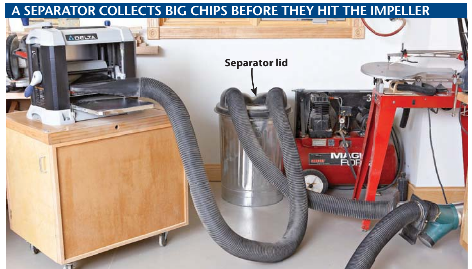
As chips fill the garbage can, collector efficiency drops, so a separator like this one needs to be emptied frequently. However, dumping sawdust from a can like this one is often easier and faster than wrestling with the collection bag of a single-stage collector.
