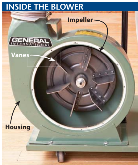
Removing a cover reveals the impeller. This one spins clockwise, pulling air and chips in, and pushing them out through the top.
