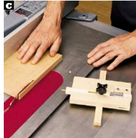
C Remove the jig before making the cut so the workpiece doesn't bind between the rip fence and the screw head. Replace the jig in the slot without making any adjustments to set up the next cut.
