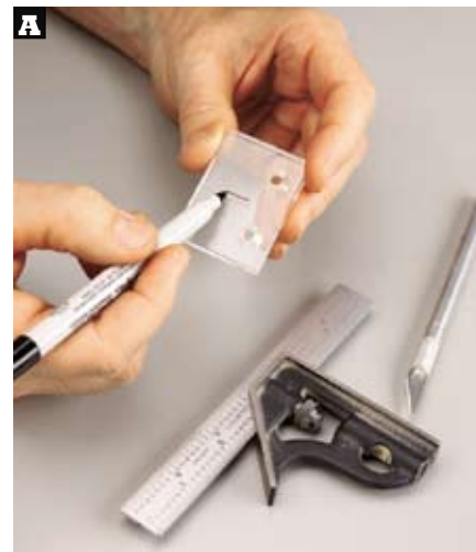
To make a cursor, scribe a line across the middle of the acrylic indicator with a sharp knife and a combination square. Color the scribed line with a permanent marker. Wipe off the excess ink with a cloth or paper towel, leaving a fine line.
