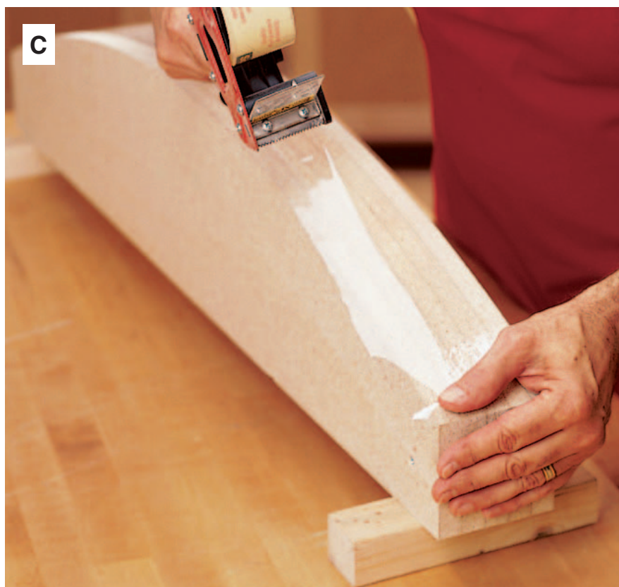
Any kind of tape will keep glue off your forms; this clear packaging tape is wide and easy to remove when you're done.
