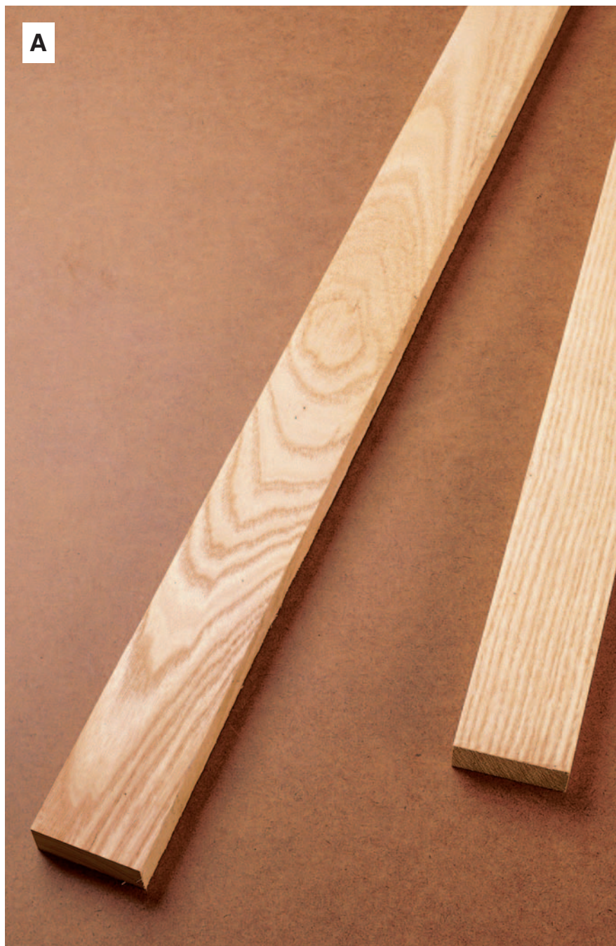
Look for bending stock with straight grain, like that on the right. When grain runs in various directions, as on the left, it’s quite likely to break.
