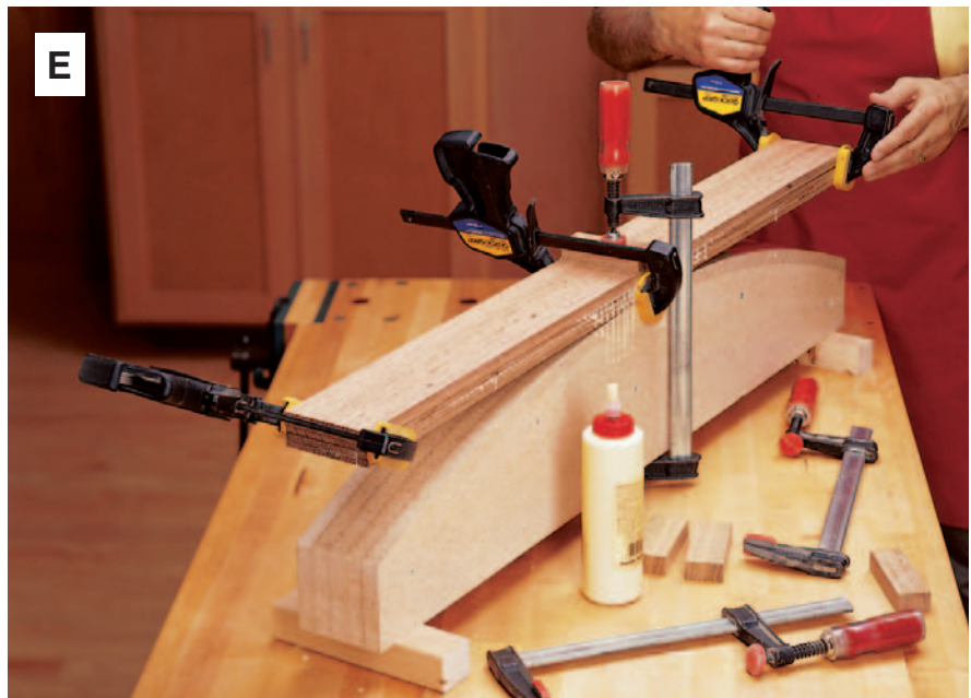
With wide, fixed jaw faces, Quick-Grip clamps do a good job of holding the strips in alignment. Place your first bending clamp right in the middle.
