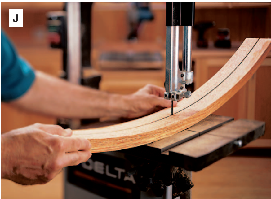
When cutting a bent lamination on the bandsaw, keep the workpiece firmly against the table at the point where the blade enters the wood.
