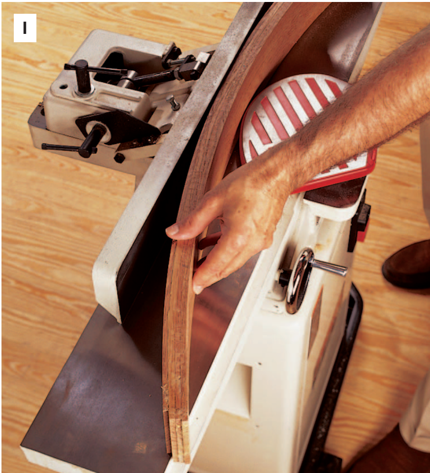
Smooth the edges of a bent lamination on your jointer. Make a test pass with the machine turned off to make sure you won't struggle with the safety guard.
