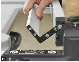
To use the rip-fence attachment, simply rotate it from the right to the left side (on most saws) and snap it into place.
