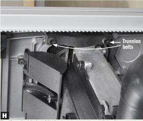
To align the blade with the top, loosen three of the four trunnion mounting bolts, and then pivot the motor/arbor assembly until the blade is within .002" of parallel to the miter slots. Then tighten the bolts.
