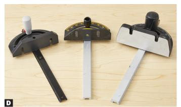
Attaching an auxiliary fence to the miter gauge on the left proves difficult because the screw slots cannot be accessed from the back side of the head. With the other two styles, you can easily screw on a plywood or MDF fence.
