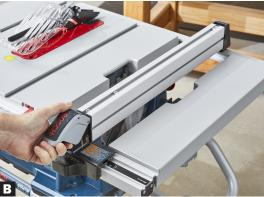
**Bosch's fence clamps to fixed rails.** To rip wider than the table size, release the lock and the small table section and rails slide in and out of the fixed rails. Also using this fence style: Ryobi RTS23 and SawStop.
