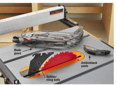
The safety guards work in four modes: blade guard and antikickback pawls mounted on the splitter/riving knife; either blade guard or pawls on the splitter/riving knife; or the splitter/riving knife by itself.
